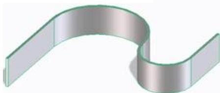
If the elements in the profile are tangentially connected, then no bend radius will be inserted between adjacent elements. If two adjacent elements are not tangentially connected, a bend radius of the specified size will be automatically entered with the new sheet metal part is created.
